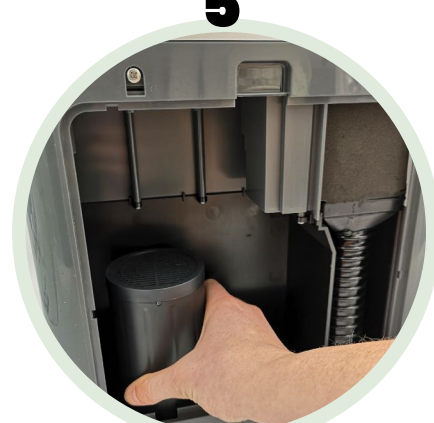
Install new filters (turning clockwise)
